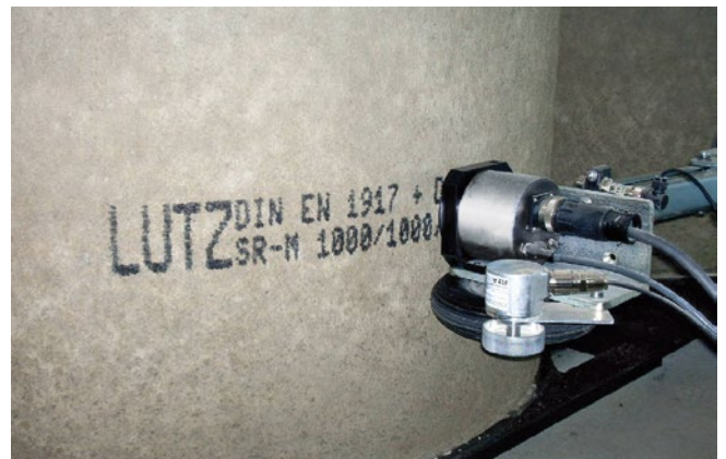
Marking of concrete pipes
